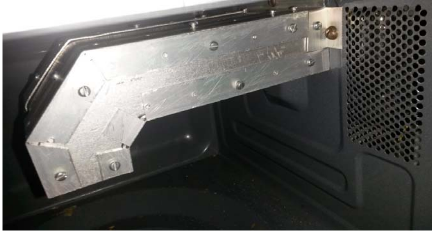
Figure 3: Implementation of waveguide into the oven cavity
