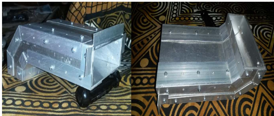
Figure 2: Waveguide with desired design
