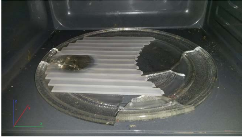
Figure 8: Melted portion of PP strips arrangement after heat treatment by modified system
