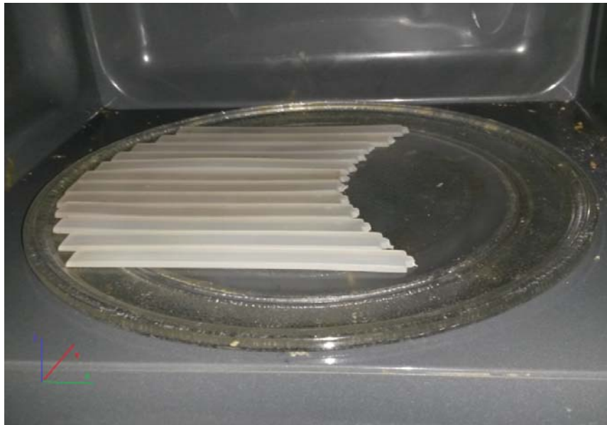
Figure 7: Arrangement of PP strip inside the oven cavity
