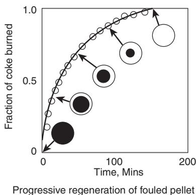
**Figure W14A-1** Shell progressive regeneration of fouled pellet. [Reprinted with permission from J. T. Richardson, *Ind. Eng. Chem. Process Des. Dev.*, 11(1), 8 (1972); copyright American Chemical Society.]
