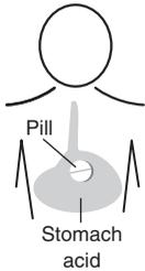
We now consider the case where the total particle is being completely consumed. We choose as an example the case where species A must diffuse to the surface to react with solid B at the liquid–solid interface. Reactions of this type are typically zero order in B and first order in A. The rate of mass transfer to the surface is equal to the rate of surface reaction.
