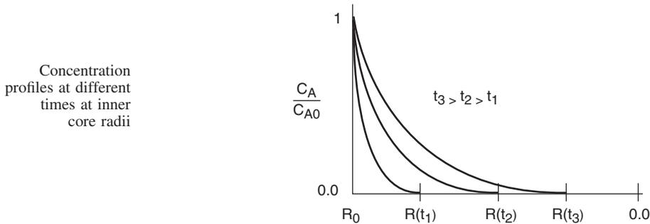
**Figure W14A-5** Oxygen concentration profile at various times. At  $t_1$ , the gas-carbon interface is located at  $R(t_1)$ ; at  $t_2$  it is located at  $R(t_2)$ .
