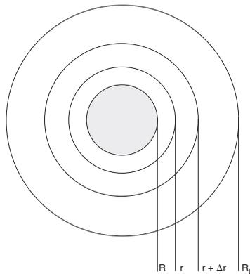
**Figure W14A-3** Sphere with unreacted carbon core of radius  $R$ .
