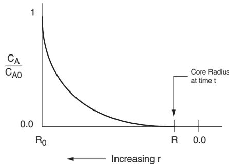
**Figure W14A-4** Oxygen concentration profile shown from the external radius of the pellet ( $R_0$ ) to the pellet center. The gas-carbon interface is located at  $R$ .
